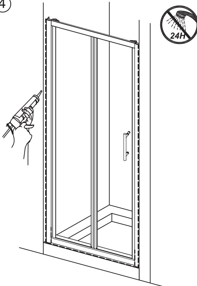
The frame drains internally. Silicone should only be applied on the outside and not to the inside of the frame.
