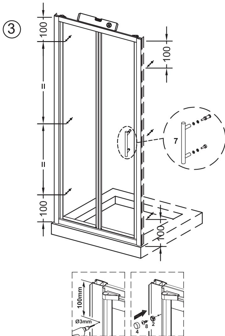
To fix the shower enclosure, check that the shower enclosure is aligned correctly.
