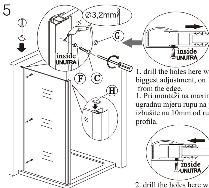
1. drill the holes here with biggest adjustment, on 10mm from the edge.
