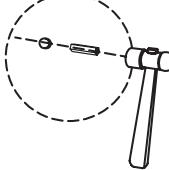
**1** Lift the shower enclosure onto the tray and mark position. Take care not to damage the tray when moving the enclosure into position. Use a spirit level, making sure the wall channels are perfectly vertical. Mark through the holes in the wall channels to drill fixing holes in the walls using 6.5 mm drill. Push the wall plugs into holes.
