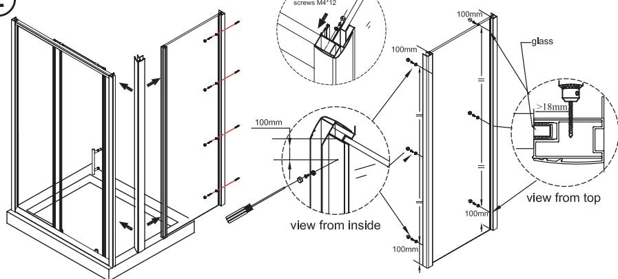
**2** Fit side panel to the wall channel using M4x30 screws and cover screws with capped washers.
