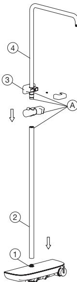
Insert the lifting rod assembly (a) into the faucet body group connector (1), ensure that the straight rod has been installed to the bottom and parallel to the wall, draw a line around the wall base (3), remove the straight rod, place the wall base group base (3) at the line drawing position, and determine the wall drilling position according to the installation hole on the base.
