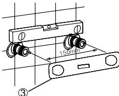
Use a level gauge (3) to confirm the distance between the joints of the two curved feet, and adjust the two curved feet to keep them horizontal.
