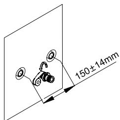
Before installation, G1 / 2 internal thread pipe fittings have been installed, with a spacing of 150mm reserved and kept horizontal. The pipe fittings shall be vertical and shall not protrude from the wall.
