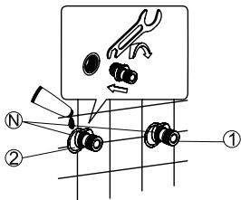
Clean the water supply channel and remove impurities in the water channel. Wrap the n-joint (2) with adhesive tape or thread sealant and screw it into the water supply pipe. After the installation is solid, the n-joint protrudes from the wall according to the scope of the clamping point of the level ruler.
