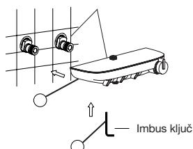
After inserting the faucet body (4) into the curved foot, make sure that the upper plane of the body is horizontal and major. The back of the body is close to the wall body (a), and then use sixTighten the inside of the faucet body with an angle wrench(5). Top wire.
