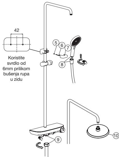
After the elbow assembly is fixed, the shower hose hexagonal connector is connected to the body connector (9), and the hose conical connector (8) is connected to the hand-held shower. **Please note** that there should be rubber gasket seals between the connectors.
