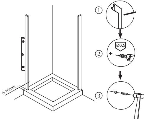
3 Fix the wall profiles to wall using screws (2). Make sure the wall profiles vertical, insert the frame into wall profiles.
