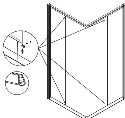
4 Fit glass clips (16), (21) to the fixed panel end. Insert fixed glass panels into upright profiles, tighten glass clips to glass using screws (18), cover screw caps (20).
