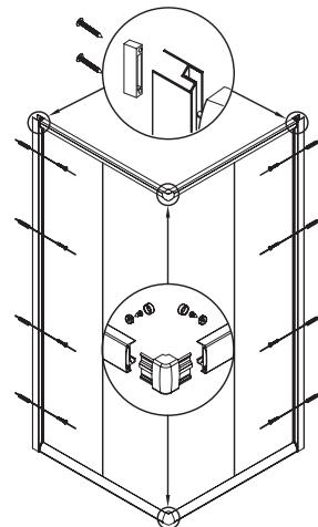
2 Connect the top, bottom tracks with upright profiles using screws (13). Join two top tracks and two bottom tracks together using corner joints and fix using screws (18).
