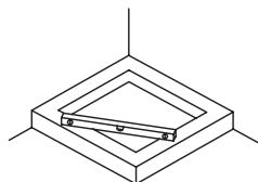
1 Adjust the tray to make it level. Drill holes onto wall according to the above right drawings and put in wall plugs.
